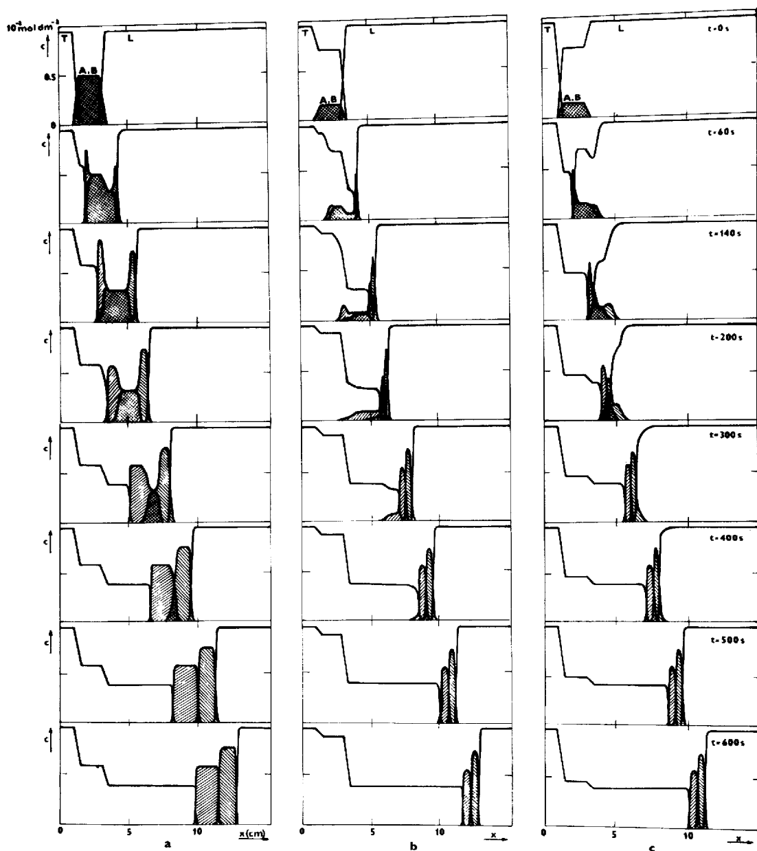
Fig. 3. Dynamics of the isotachopheretics separation for: (a) sampling through a valve into the free space between the leading and terminating electrolyte; (b) sampling with a syringe before the boundary into the terminating electrolyte; (c) sampling with a syringe behind the boundary into the leading electrolyte.
